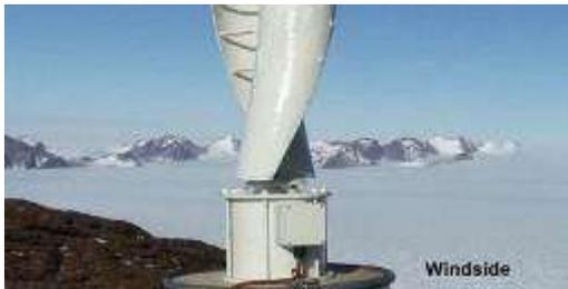
Savonius, Bi-Conical or Helical, Vertical Axis Wind Turbine
